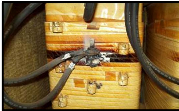
Burned Out Transformer Core
